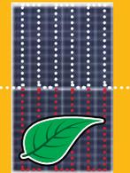
With the same shading, an REC TwinPeak module has more surface area still producing electricity.
