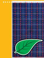
When one half of a standard module is shaded, none of the module produces electricity
